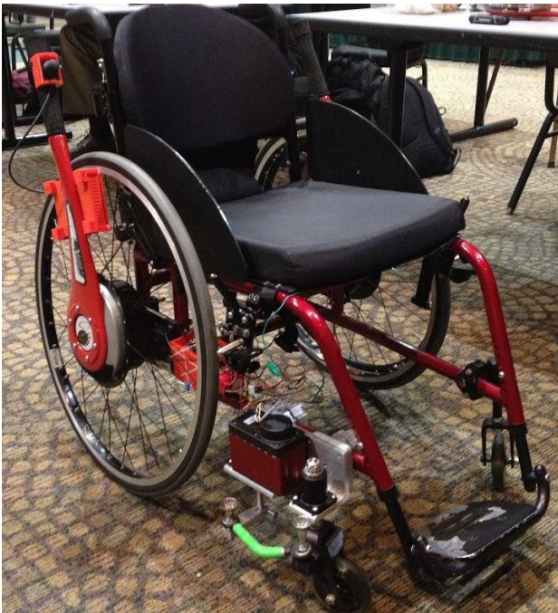
Fig. 5. Wijit Lever System [13]
