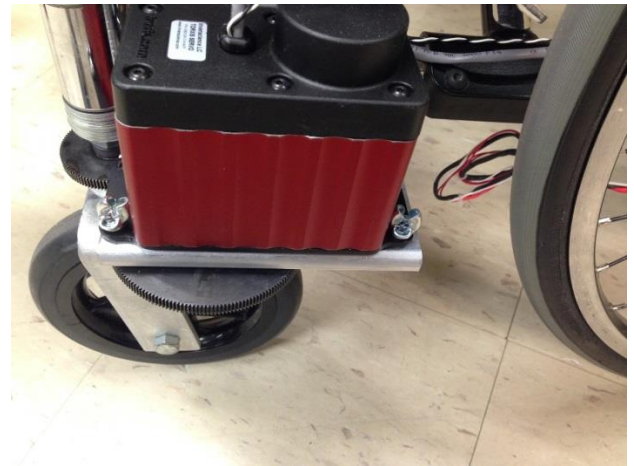
Fig. 17. Negative/Reverse Caster Position [13]
